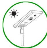
2nd Step: The solar lamp will be off at daytime and start charging when the solar voltage more than 5v.
