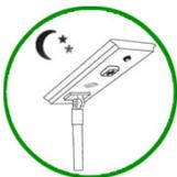
3rd Step: With the light sensor function, the LED lamp will auto turn on at dusk. It is 30% brightness when standby(if with motion sensor).
