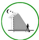
5th Step: If there is no continue movement detected within the sensor area after 30s, it will be standby mode again to save power. The delay time and brightness can be customized.
