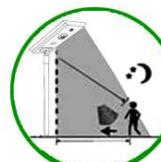
4th Step: When movement detected, it will switch to 100% brightness for 30s.
