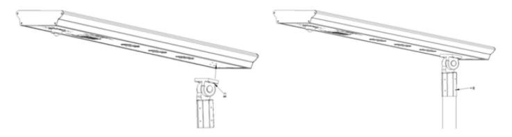
Use 4 screws to fix the fitting support on the lamp and fix the lamp on the pole with screws.
