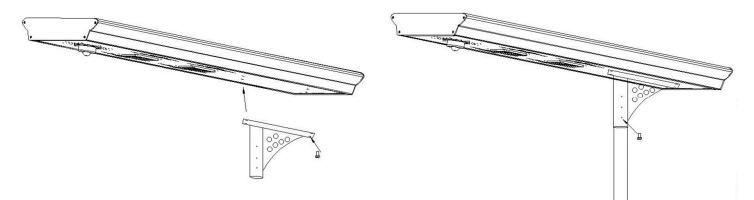
Use 4 screws to fix the fitting support on the lamp and fix the lamp on the pole with screws.
